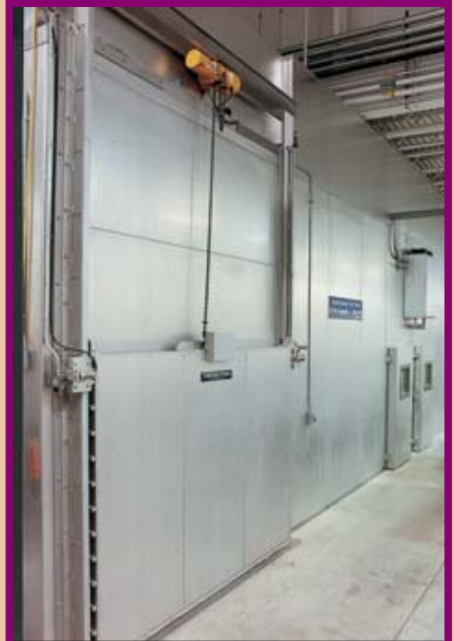
This two-room walk-in chamber efficiently tests the performance and reliability of air-conditioning units.
